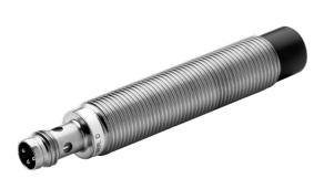
Inductive Proximity Sensor, 3-Wire DC, Short Barrel, 12mm Diameter, Tubular:Nickel Plated Brass, Short, 4mm Sensing Distance, Unshielded, N.O., Source (PNP) Output, Micro QD (DC)
